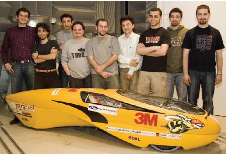
METYX Composites provided specialty non-crimp reinforcements made out of high tenacity carbon and aramid fibers as well as low density structural foams. Thanks to the materials the body was lightweight and durable. The vehicle performed well in the competition, ranking 16th and traveling a distance of 551 kilometers on only one liter of fuel!
