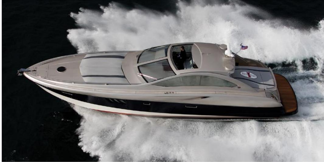
*“METYX Composites produced custom METYCORE reinforcements for this demanding RTM application. Series production for the elite 55 foot super yacht, which integrates this high-tech hard top, is still going at full speed.”*
